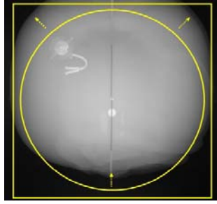
Fig. 4 Upward distortion of propagating flame affected by buoyancy
